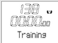
Once you are in the menu **Training**, your HR monitor automatically switches to the main display. This displays the already recorded training time on the middle line (after Save/Delete: 00:00:00) and on the line below **Start**.
